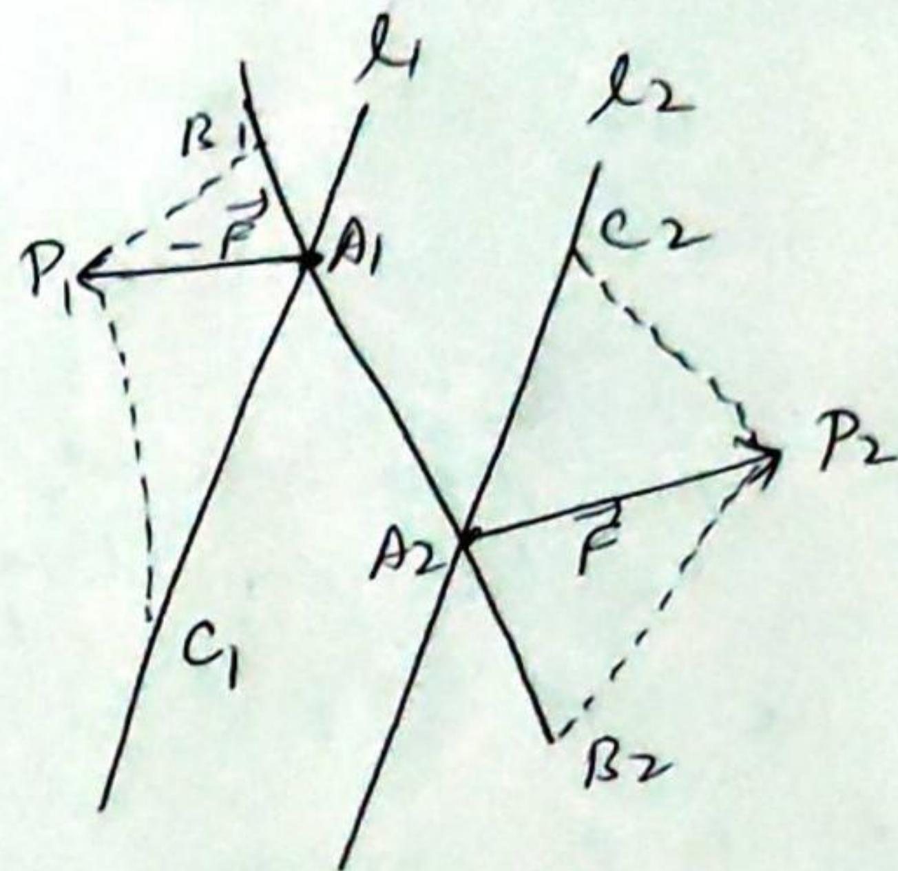
Draw the parallelogram  $A_1 B_1 P_1 C_1, A_2 B_2 P_2 C_2$  having  $A_1 P_1, A_2 P_2$  as diagonals and the sides being parallel to  $A_1 A_2$  and  $l_1$ .
