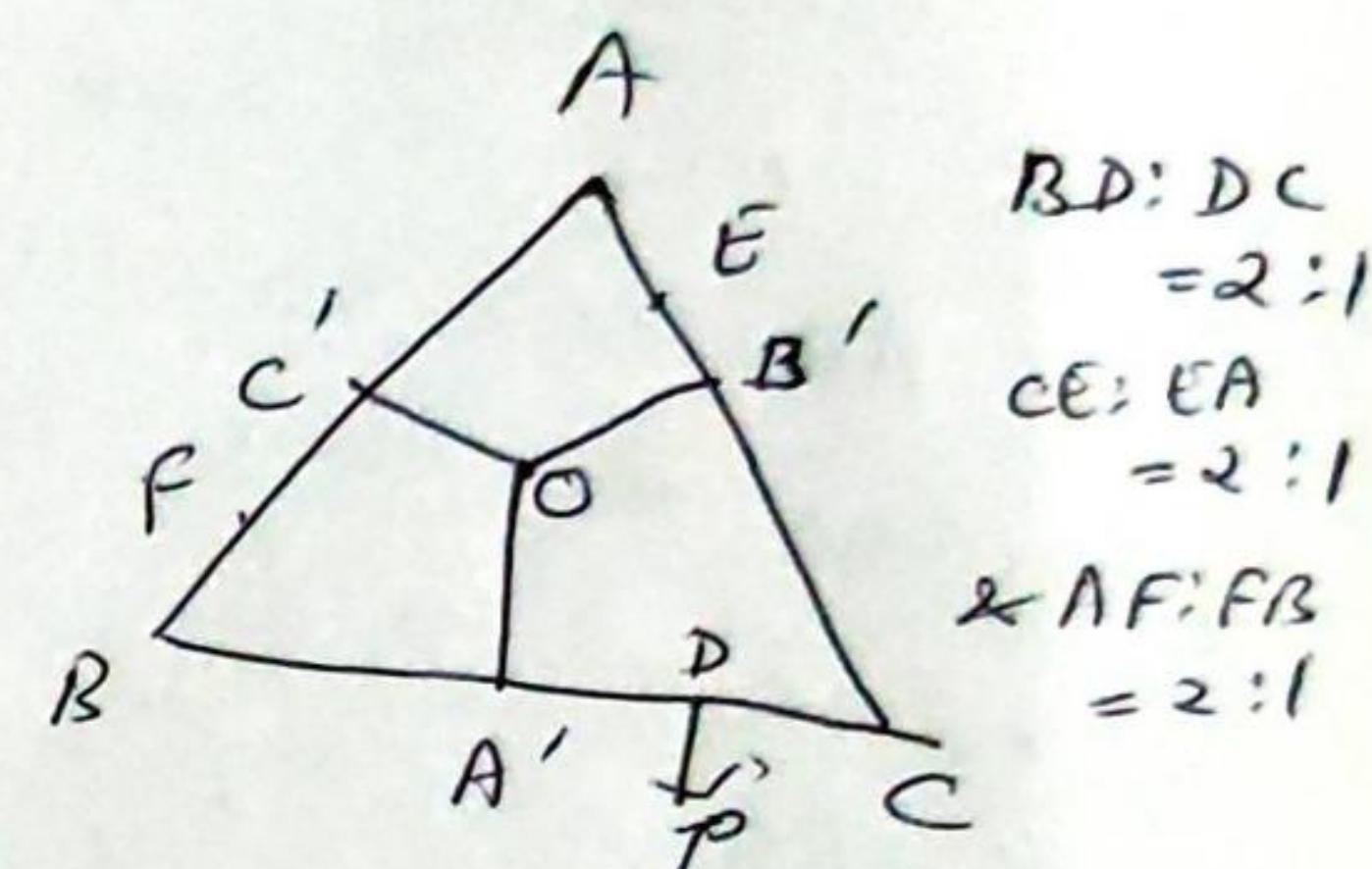
The three equal forces  $P$  acting at  $O$  & to the sides of the triangle are in equilibrium by the perpendicular triangle of forces.
